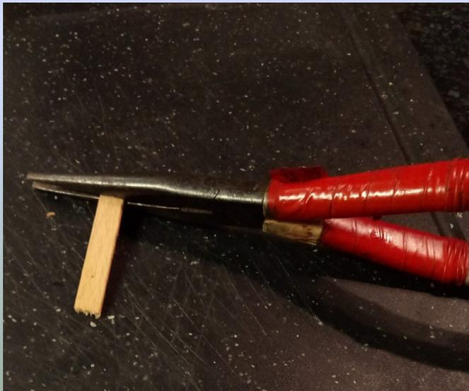
Break the wooden stick to the desired length. You can easily break small pieces with pliers.
