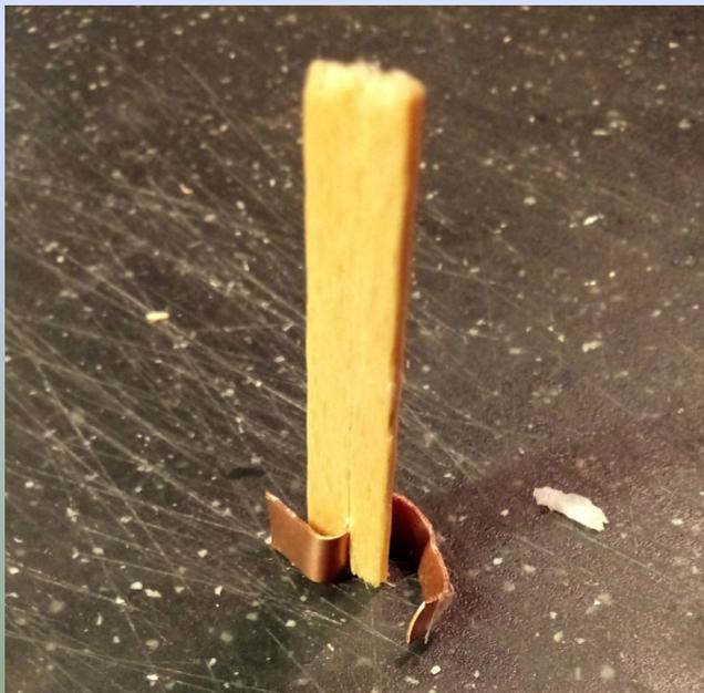
Insert a small sheet of metal into the gap.
